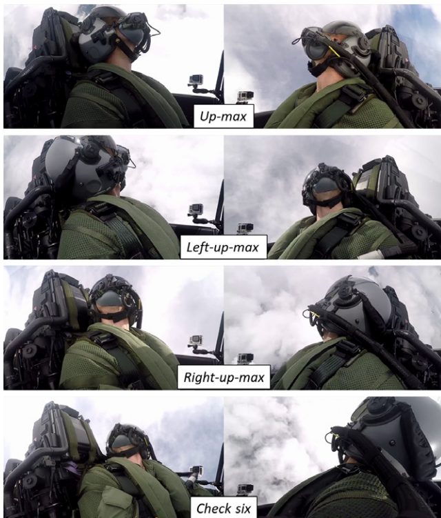
Fig. 1. Pictures of the left and right front perspectives of the GoPro cameras showing the scripted head movements (up-max, left-up-max, right-up-max, and check six).
