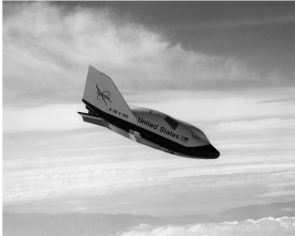
Fig. 4. X-38 CRV in drop tests in 1998 (courtesy of NASA).
