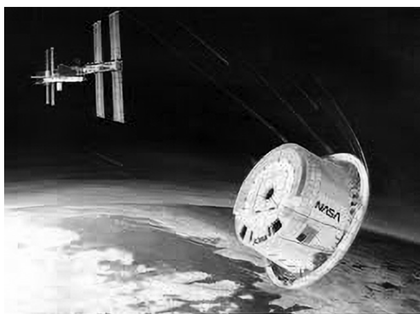
Fig. 2. SCRAM (ballistic ACRV) as envisioned by NASA in 1993 (courtesy of NASA).
