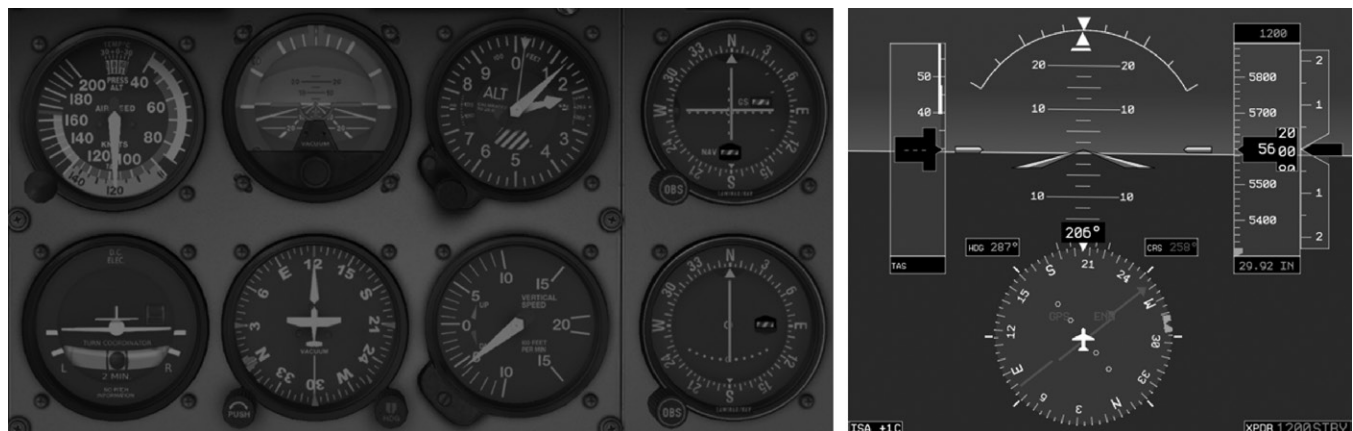
Fig. 1. Comparison of legacy steam gauge blind flying panel to attitude display indicator and horizontal situation indicator.
