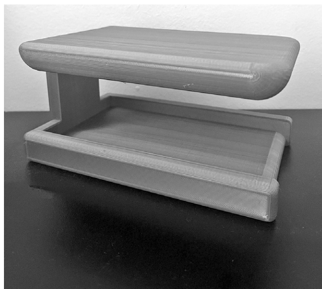
Fig. 1. Original sterilizer 3D-printed via the Autodesk Fusion 360 program.
