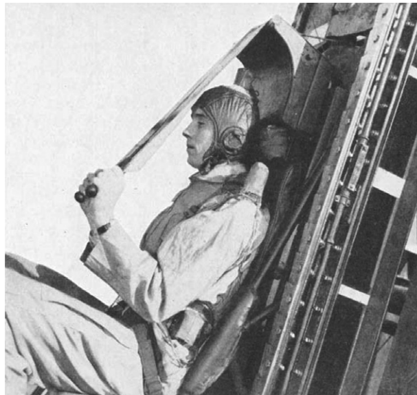
Fig. 1. "Subject in correct position preparatory to reaching for firing curtain. Accelerometers can be seen on the hip, shoulder, and head."
