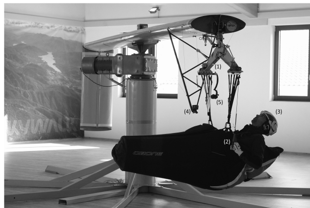
Fig. 3. Participant in recumbent ('cocoon') harness in spiral configuration, looking up at the LED lights (1), with hands in the brake lines wearing standard gloves (2) and helmet (3) being filmed by cameras in wide view (4) and close-up handle view (5).
