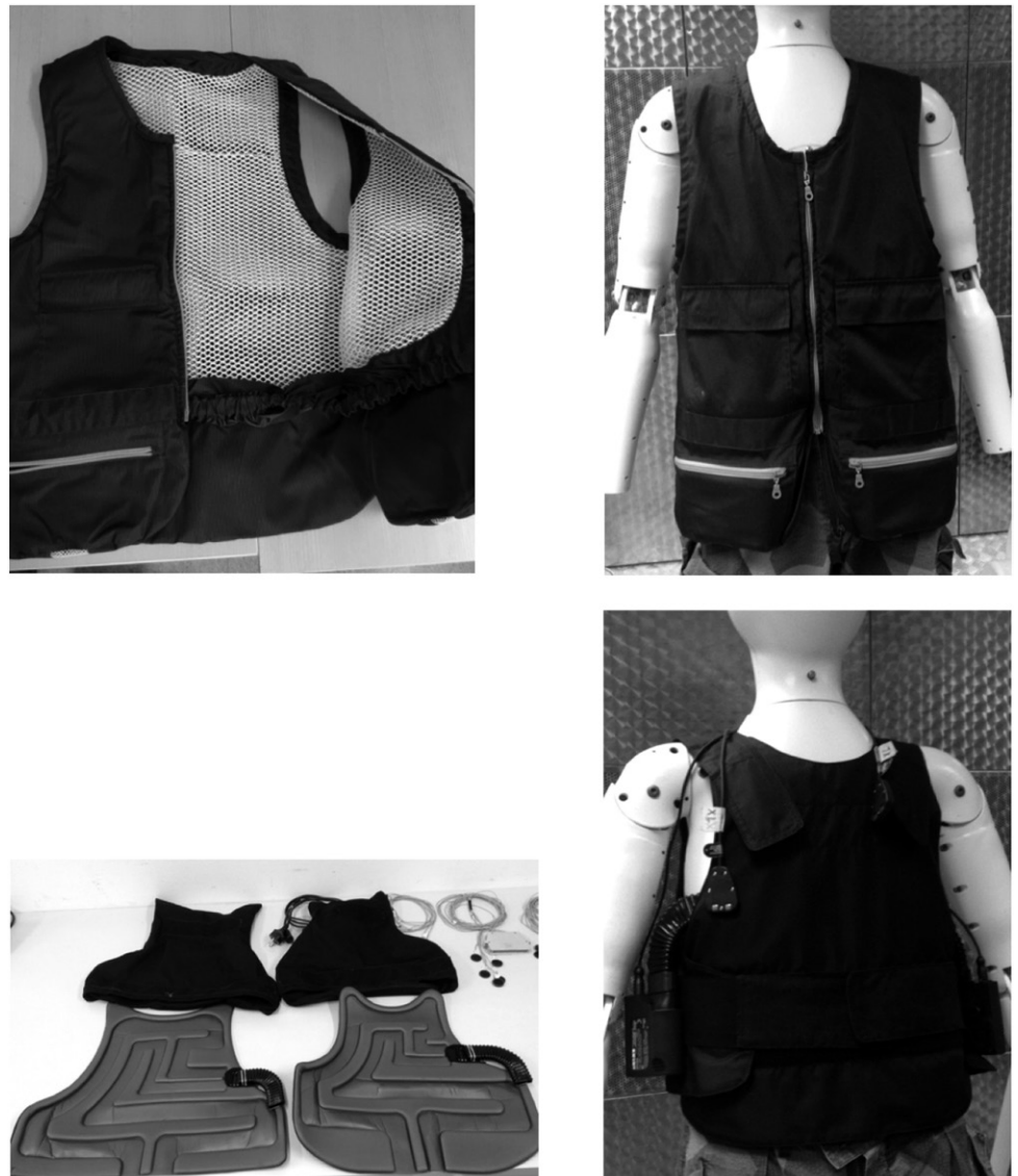
Fig. 1. The upper panel shows the Vent-1 vest (Entrak) and the lower panel the Vent-2 vest (Hexonia). In each panel, the left photo reveals the internal structure of the vest and the right photo the vest donned on the thermal manikin.
