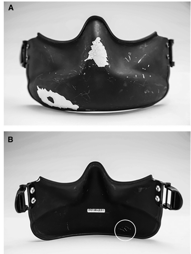
Fig. 2. MFS worn by OH-58D pilot during mishap. A) Front side of the MFS with chipped paint indicating impact locations over the areas protecting the nose and right mandible. B) Back side of the MFS with slight paint chipping on the interior surface protecting the right mandible (image bottom left).
