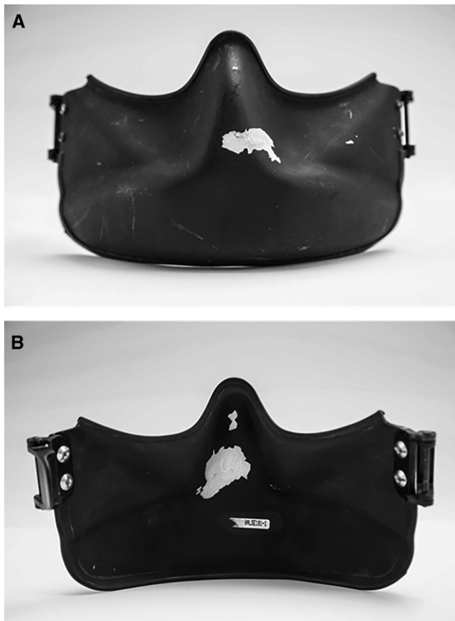
Fig. 3. MFS worn by CH-47F crewmember struck by dislodged maintenance panel. A) Front side of the MFS with chipped paint and material damage at the impact location over the area protecting the maxillary region. B) Back side of MFS with chipped paint and material damage on the interior surface the impact location.
