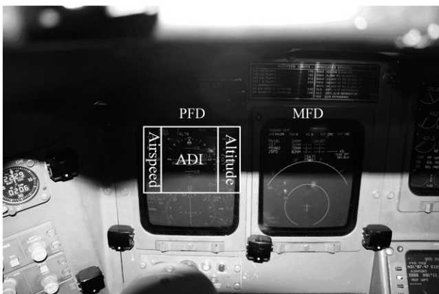
Fig. 2. The Primary Flight Display (PFD), Multi-Function Display (MFD), and three areas of interest (AOIs).
