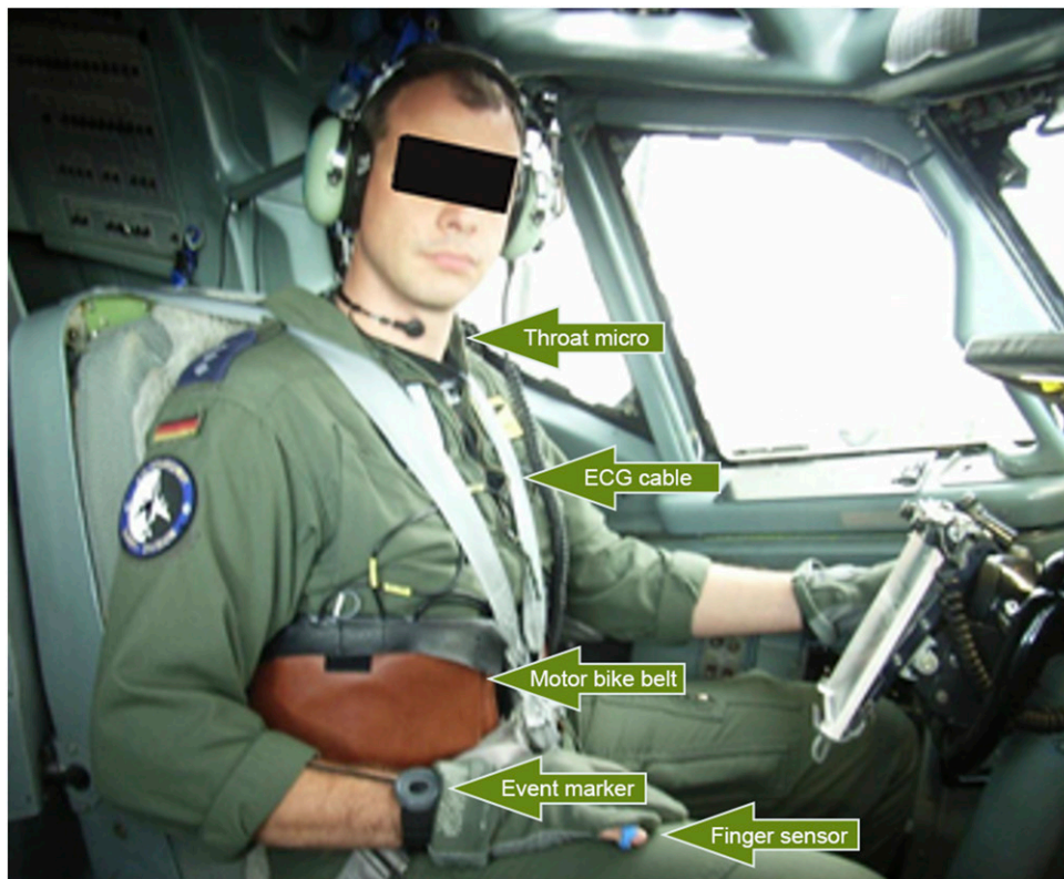
Fig. 1. Measurement equipment during simulator and real flights.
