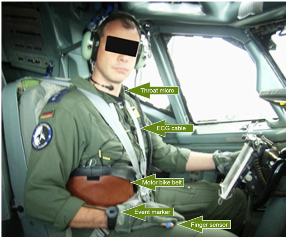
Fig. 1. Measurement equipment during simulator and real flights.
