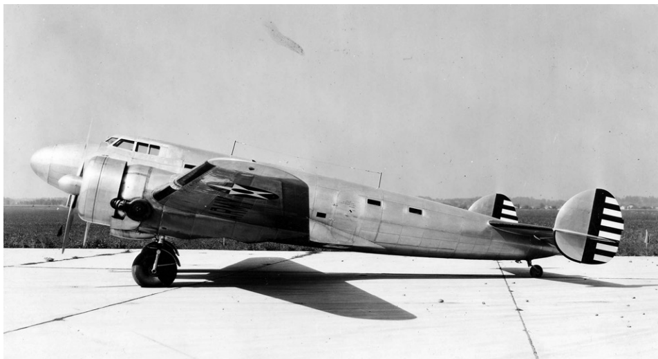
Fig. 1. Lockheed XC-35. Note the small cockpit and cabin windows which were easier to build strong enough to withstand cabin pressurization (although the entrance door and easiest to see last two windows are in the non-pressurized aft section of the plane). Additionally, notice the circular-shaped turbosupercharger on the side of the engine that forced more air into the engine, improving high altitude performance and also provided compressed air for cabin pressurization.
