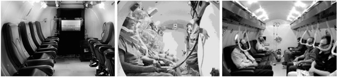
Fig. 2. Typical two-row seating configurations in a cylindrical chamber having a shared television screen (left). Patients breathing via a hood (middle) and masks (right).
