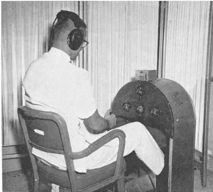
Fig. 1. Simulated pilot operation. Task consists of cockpit-like console with a stick, rudder pedals, and a throttle quadrant control.
