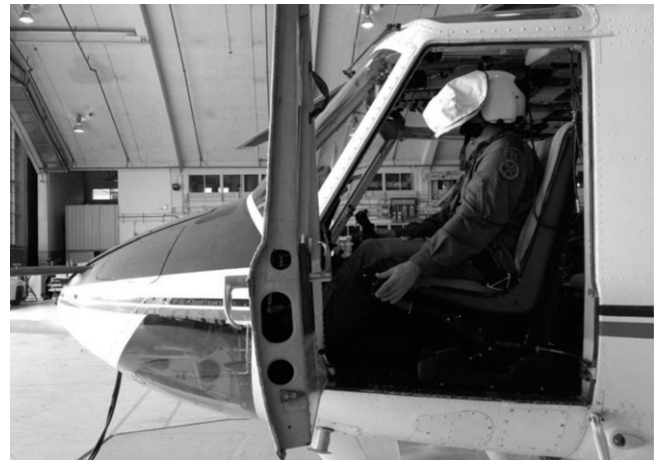
Fig. 1. The blind flying hood attached to the flight helmet (completely obscured the subject's external vision), with the subject seated in the left seat of the NRC ASRA.
