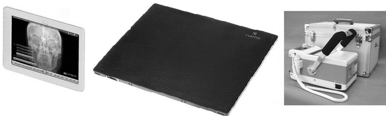
Fig. 1. Portable radiography setup: high definition tablet display (left), direct digital TFT X-ray receptor (middle), and portable generator (right).
