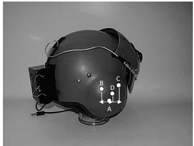
Fig. 1. The centers of mass of the various helmet configurations used by helicopter aircrew: A) the head, alone; B) the helmet alone; C) NVG; D) NVGcw. From Forde et al. (28); reproduced with permission from the authors.
